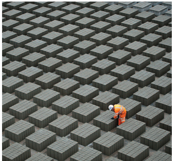
Lightweight and dense precast concrete blocks contain recycled content including fly ash and crushed demolition waste.
